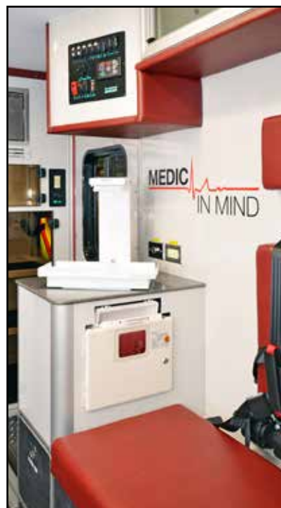
Medic in Mind layout at head of squad bench has duplicate controls and equipment on right side – everything within arm's reach.
